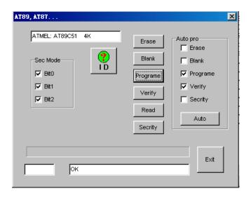
2 Write the component, Especially pay attention to the component model, before writing the component. After no mistake is confirmed in all device. Put the programming component on the outlet lock slat.
