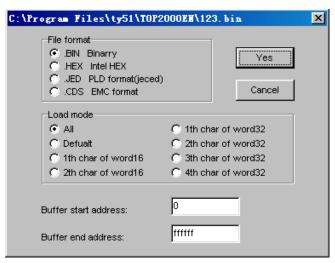
The data is loaded into the buffer area after confirming the file format. And start address. Display as follows.
