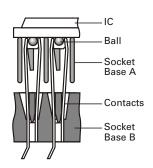
Since the solder balls are touched by two contacts on each side, the solder ball damage can be minimized; additional features are low actuation force and compact socket size
